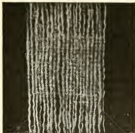
Fig. 9. Half-linen goods subjected to sulphuric acid test. Linen remains; cotton is almost entirely dissolved. Mag. 4x.
